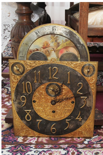
Dial As Found and After Resilver of Chapter Ring and Brass Cleaning
