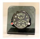
Mike Klevickis brought 2 Soviet era clocks. On the left is a clock from their MIG fighters that was used to coordinate flight operations and fuel consumption. They used a mechanical clock in order to avoid disruption from an electro-mechanical pulse from a potential atomic weapon. It could also survive the effects of an 8.5G aeronautic maneuver with accuracy. On the left is a doomsday clock used in the ICBM missiles.
